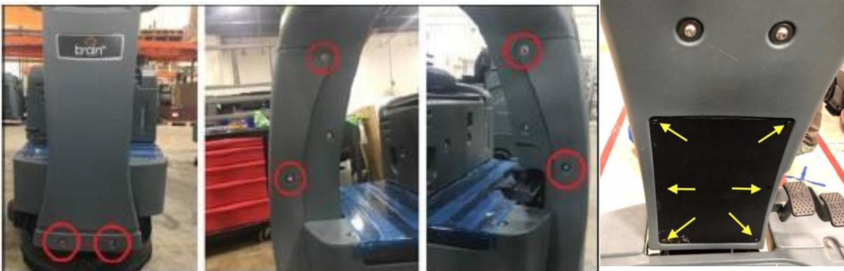
**Figure 3: Removing both access panels**
