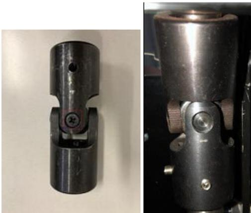
**Figure 1: Example of a U-joint in good condition**
