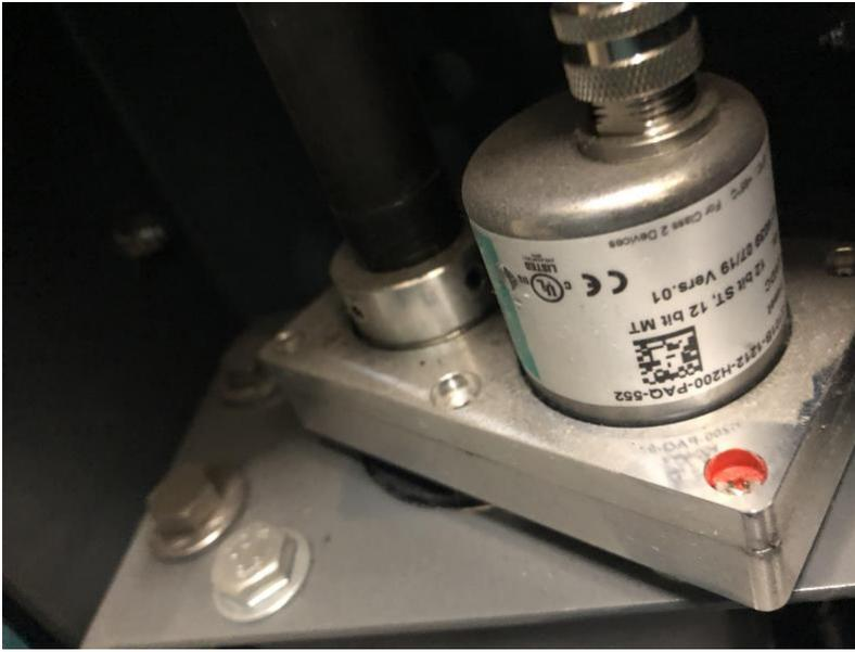
**Figure 6: Steering encoder not properly mounted**
