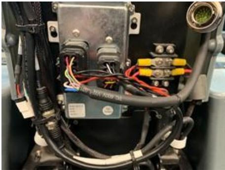
**Figure 7: Example of a steering amplifier in good condition**
