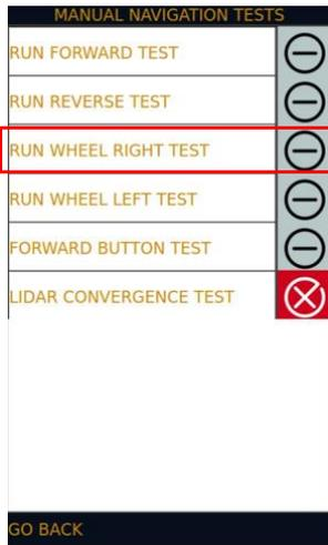
**Figure 21: Run Wheel Right Test**
